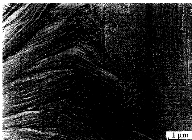
Figure 14 Transmission electron micrograph of replicates of a homopolymer sample treated with permanganic acid. The sample was obtained from the bulk of a melt-crystallized sample
